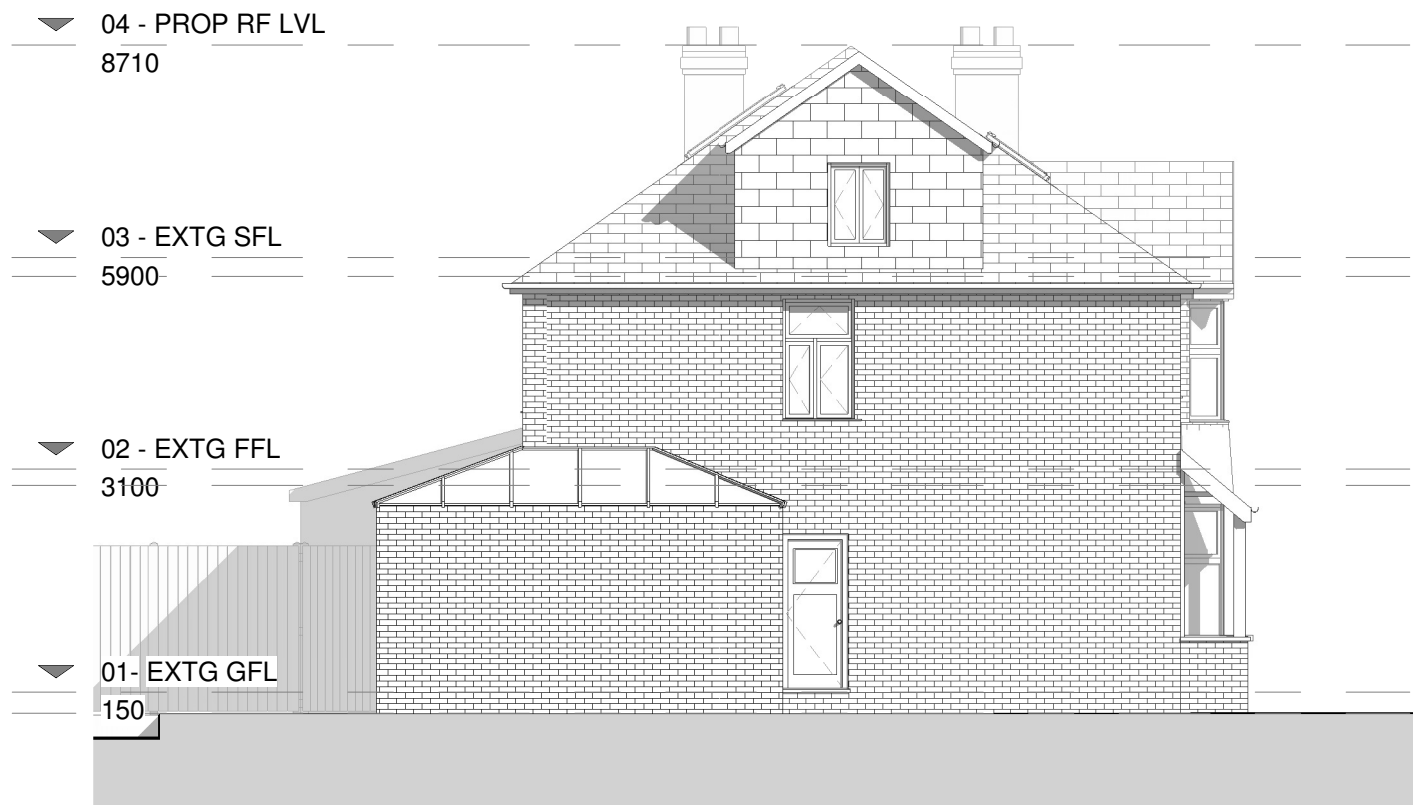
Existing Side Elevation 1 : 100
