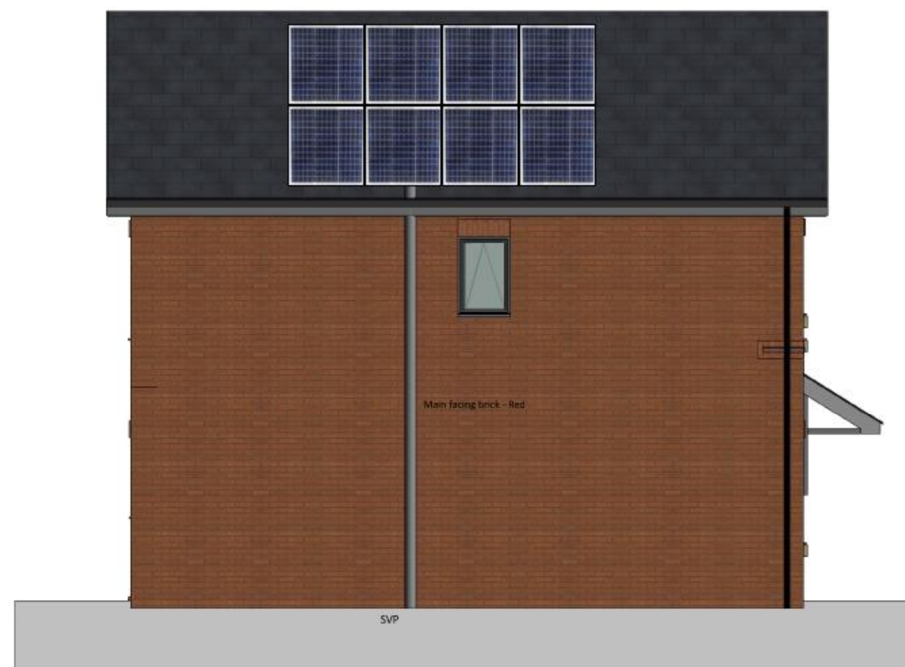
Gable Elevation - 2 Brick Type A 1 : 50
