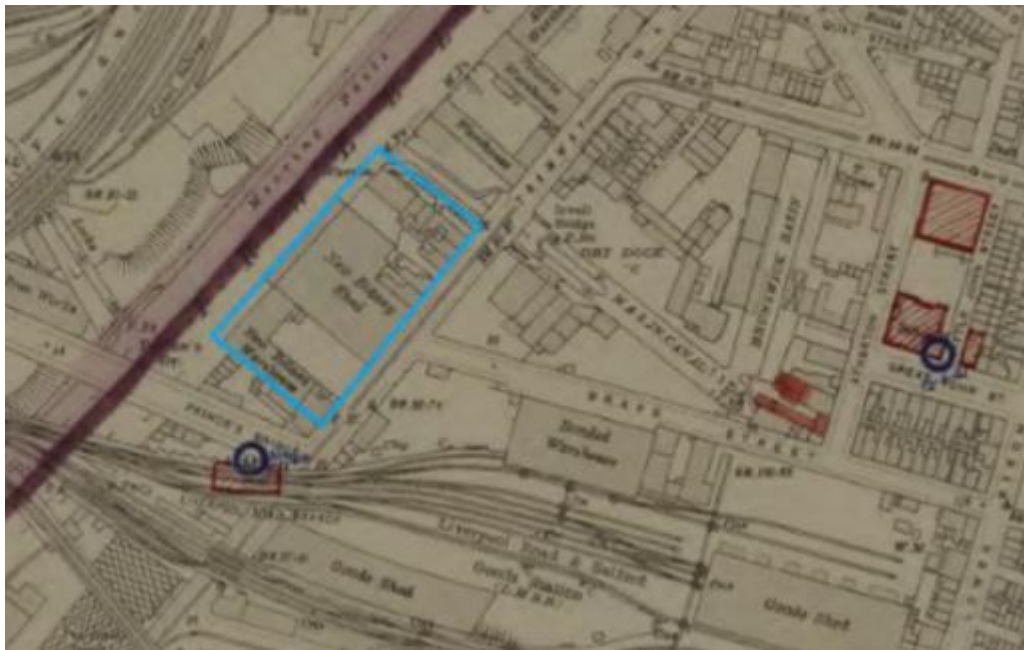
Figure 2.5: Site boundary shown in light blue. Blue circles represent high-explosive bomb hits. Pink shading for demolished buildings, lines mark bomb damage during the Blitz.
