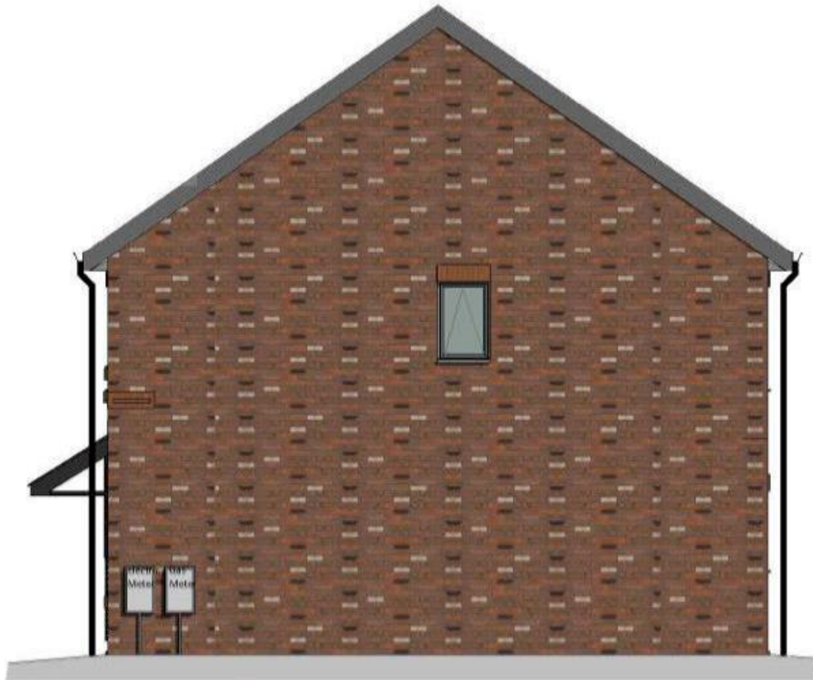
Gable Elevation (Pitched Roof) Brick Type B 1 : 50
