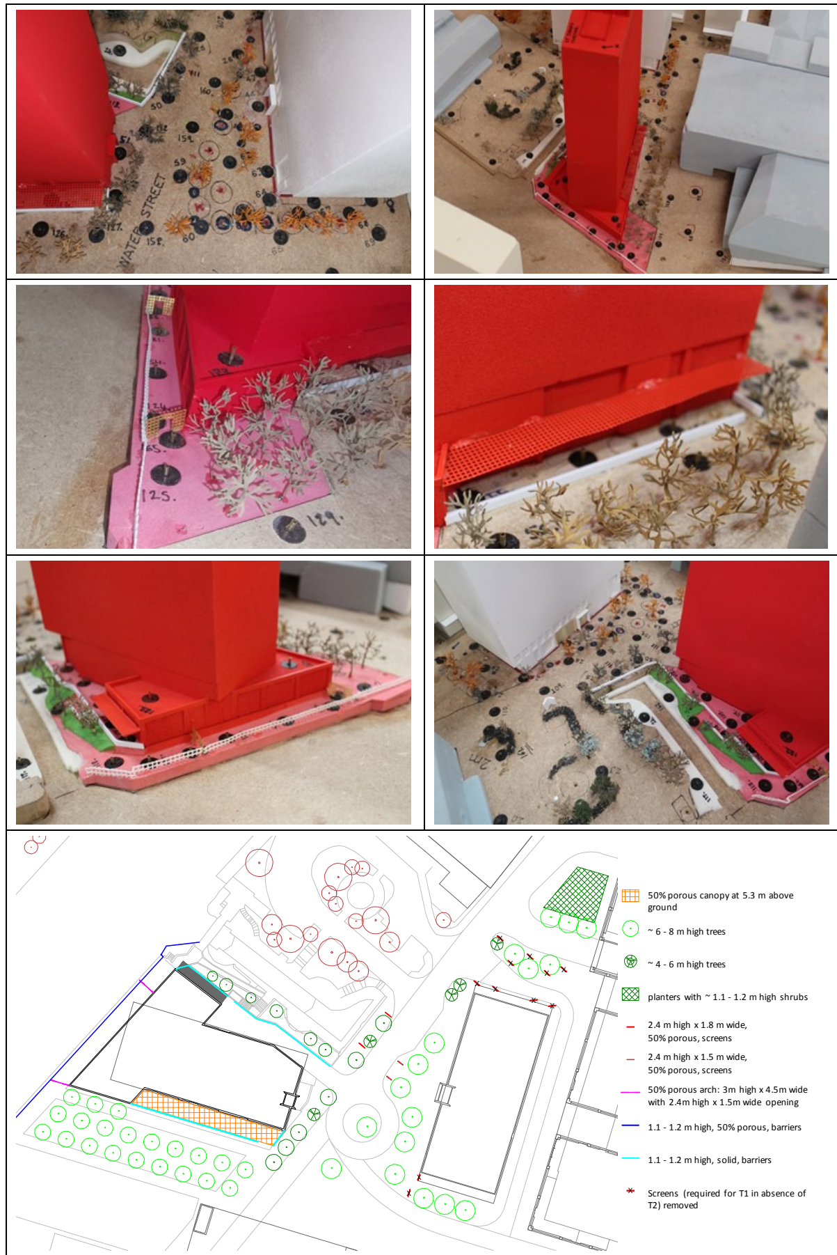
Figure A.2b: Wind Tunnel Models (Designed-In Features and Landscaping)
