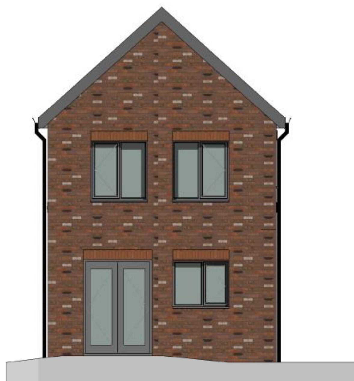
Rear Elevation Brick Type B 1 : 50
