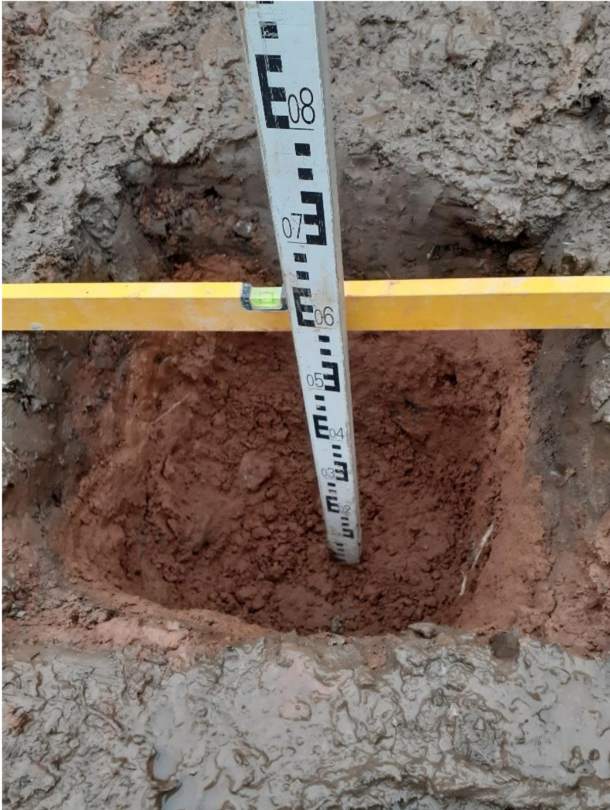
Photograph 3 Plot 5 showing 200mm of topsoil and 400mm of subsoil.
