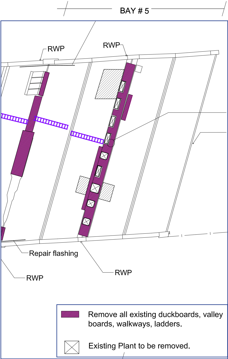
Extract from approved drawing SDA Dwg 261/PD/214 works to roof plan showing M&E units in the valley to be removed.
