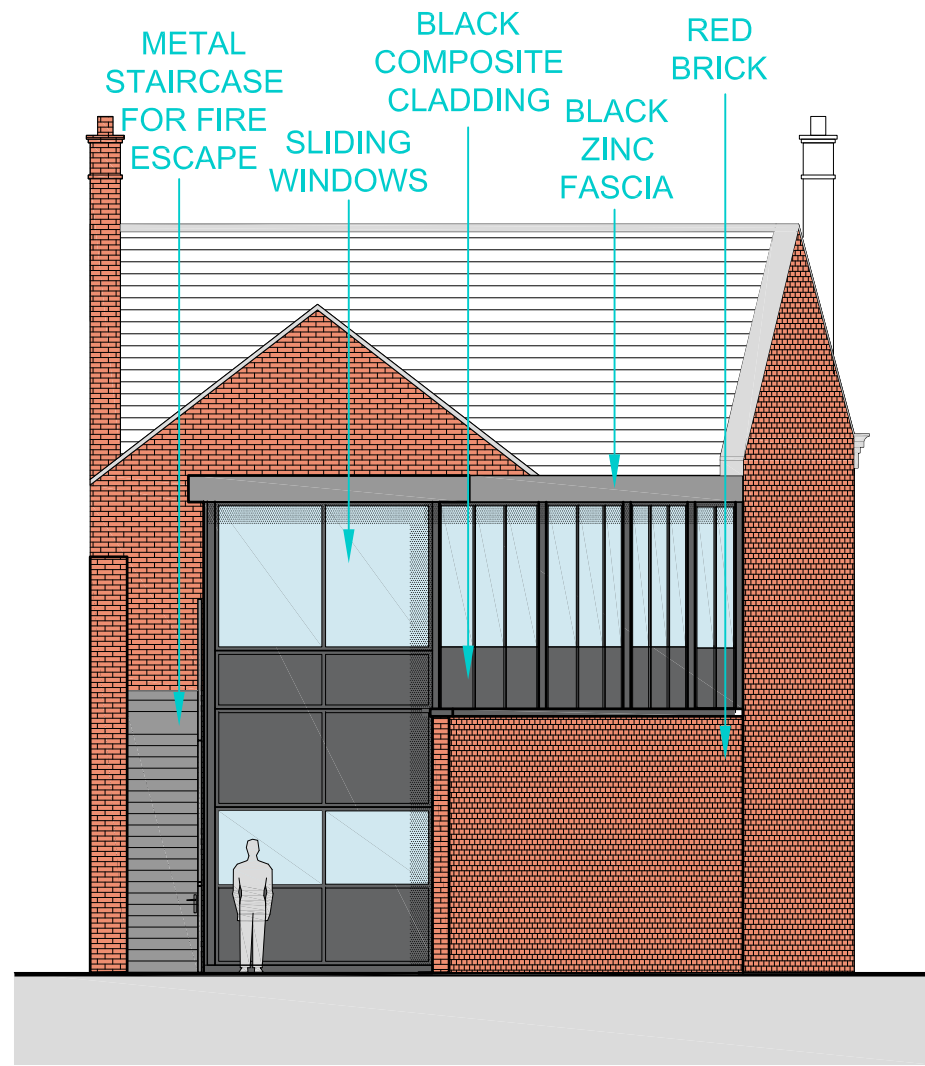
AS-BUILT REAR SECTIONAL ELEVATION Scale 1:100@A1
