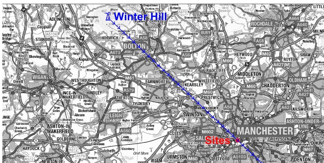
Figure 8 - The Locations of the Winter Hill Transmitter, the Sites and the direction of the incoming DTT signals at the Sites (indicated by the blue arrowed line)
