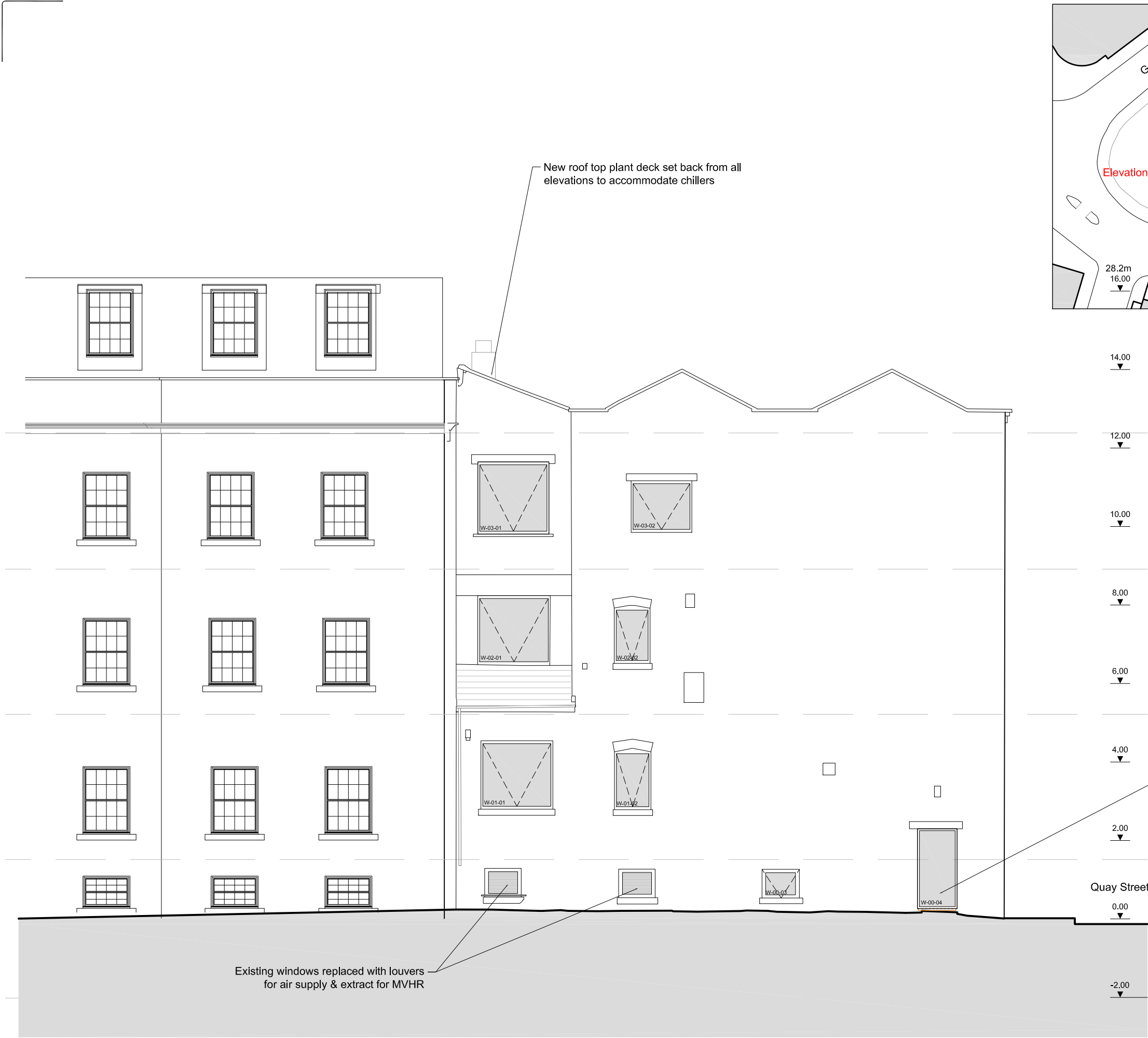
Side Elevation facing Gartside Street
