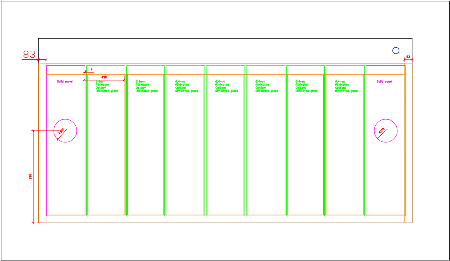
Plan with glazing and solid panels
