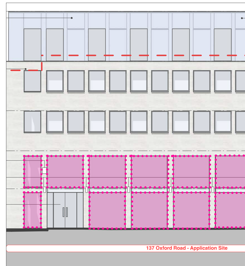
New Ground Floor Front Glazing
