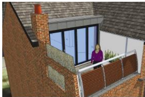
Approved balustrade and privacy screen arrangement
