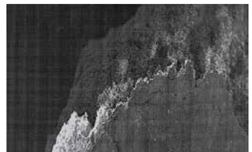
Electron microscope scan: White areas: latent hydraulic compounds which penetrated into the pore structure of the substrate – and reacted to form a pore blocking crystal.
