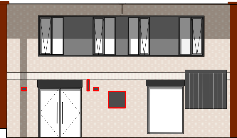
External elevation - signage and air bricks highlighted
