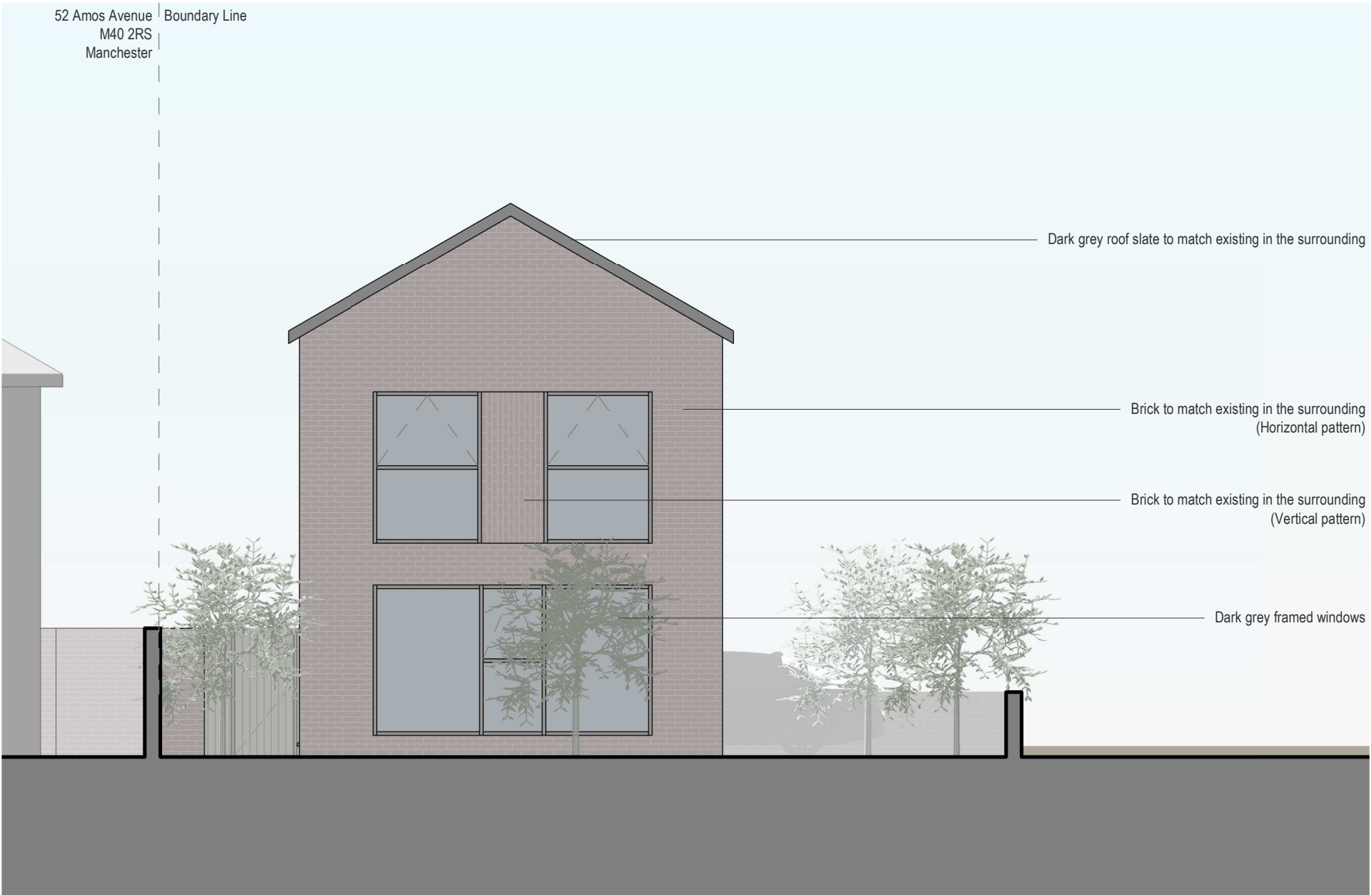
01 PROPOSED ELEVATIONS - NORTH (FRONT ELEVATION - AMOS AVE) 1 : 75
