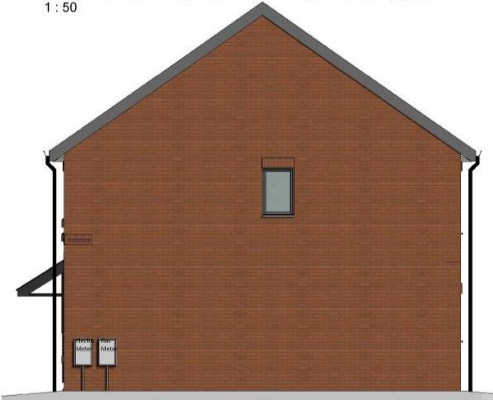
Gable Elevation (Pitched Roof) Brick Type A 1 : 50
