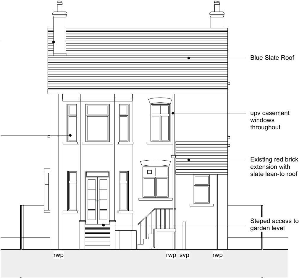
Existing Rear Elevation (South) 1:100
