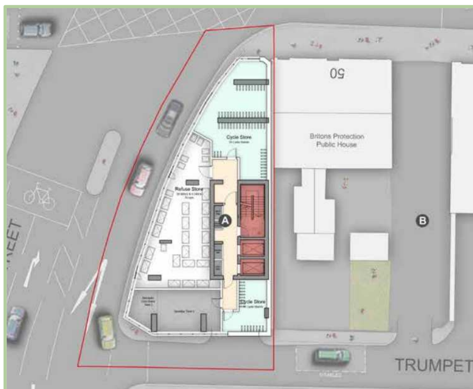
Figure 4.10 – Cycle Storage on First Floor (Site A)
