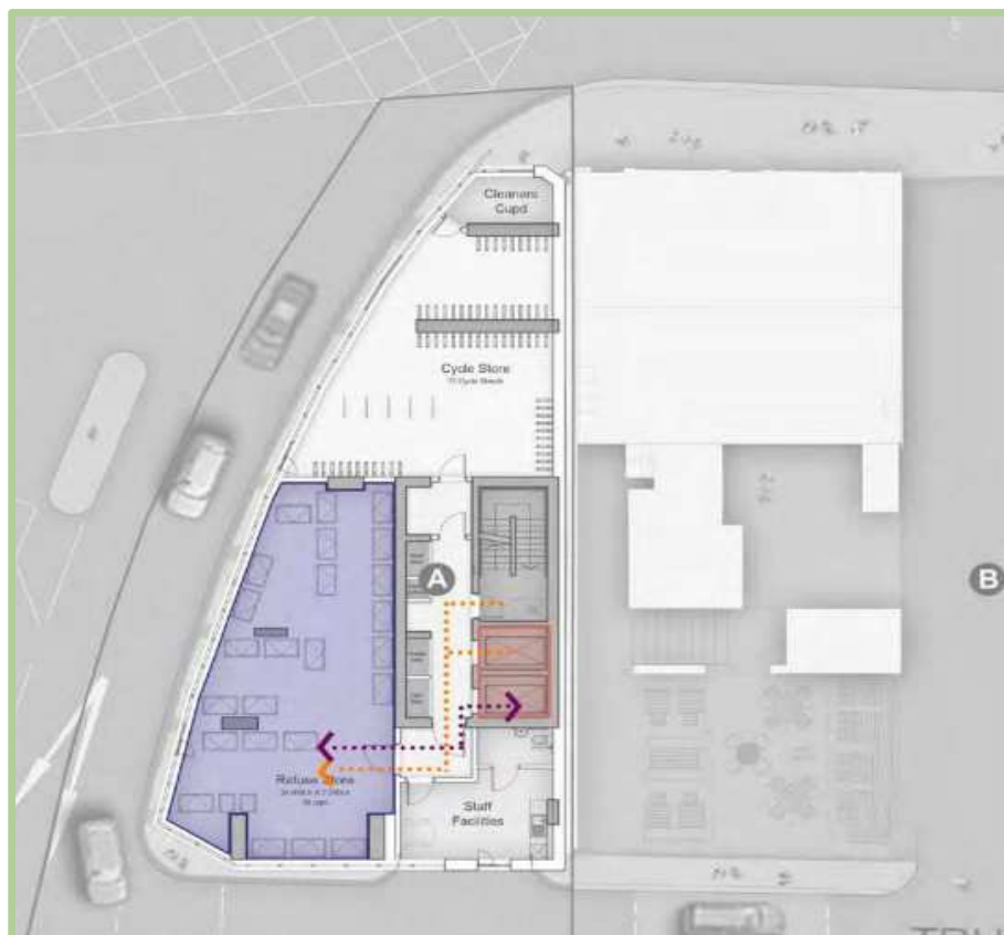
Figure 4.10 – Refuse Store on First Floor (Site A)
