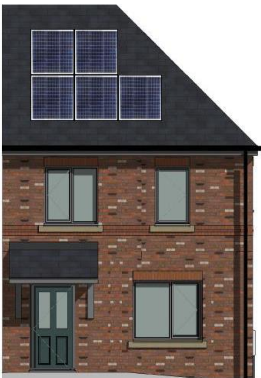
10 Front Elevation - Brick Type B Hipped Roof 1 : 50
