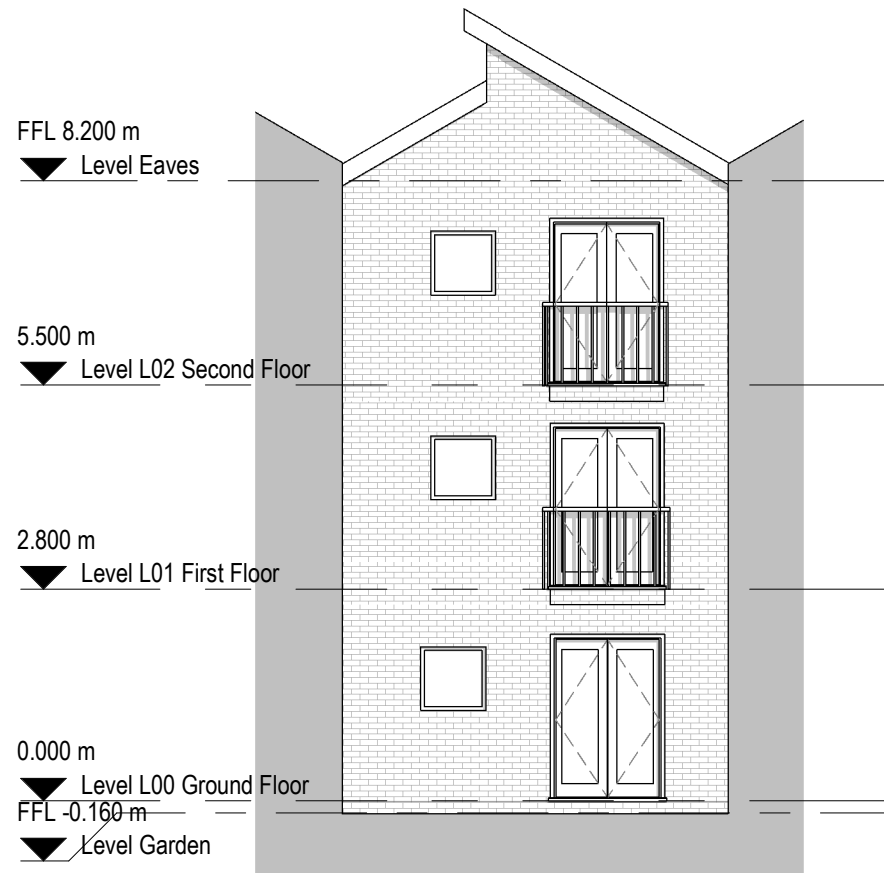
3 Existing North Elevation 1 : 100
