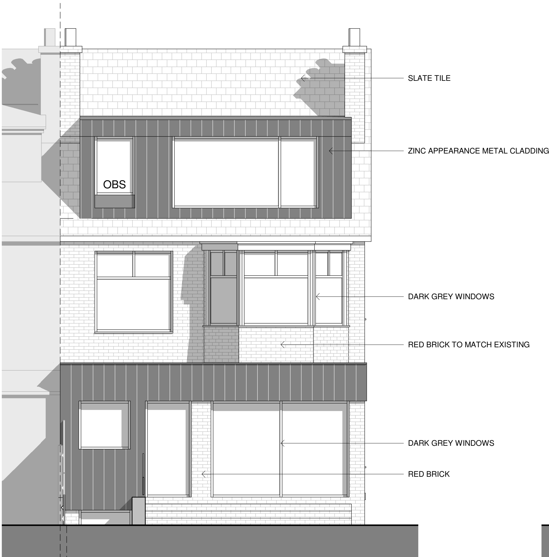
PROPOSED ELEVATIONS - NORTH-WEST 1 : 50
