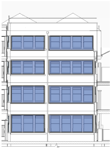
Existing Internal facing lightwell windows to be upgraded to timber frame and double glazing.
