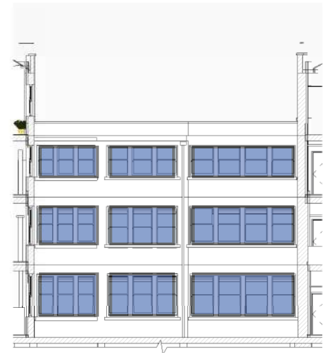
Existing Internal facing lightwell windows to be upgraded to timber frame and double glazing.
