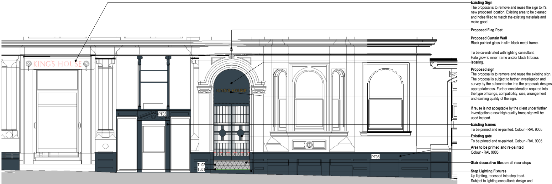
North Elevation External Glazing & Finishes 1 : 50
