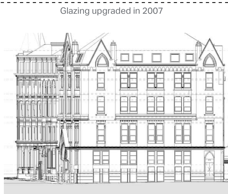
Existing Butter Lane Elevation showing the windows that were upgraded in 2007
