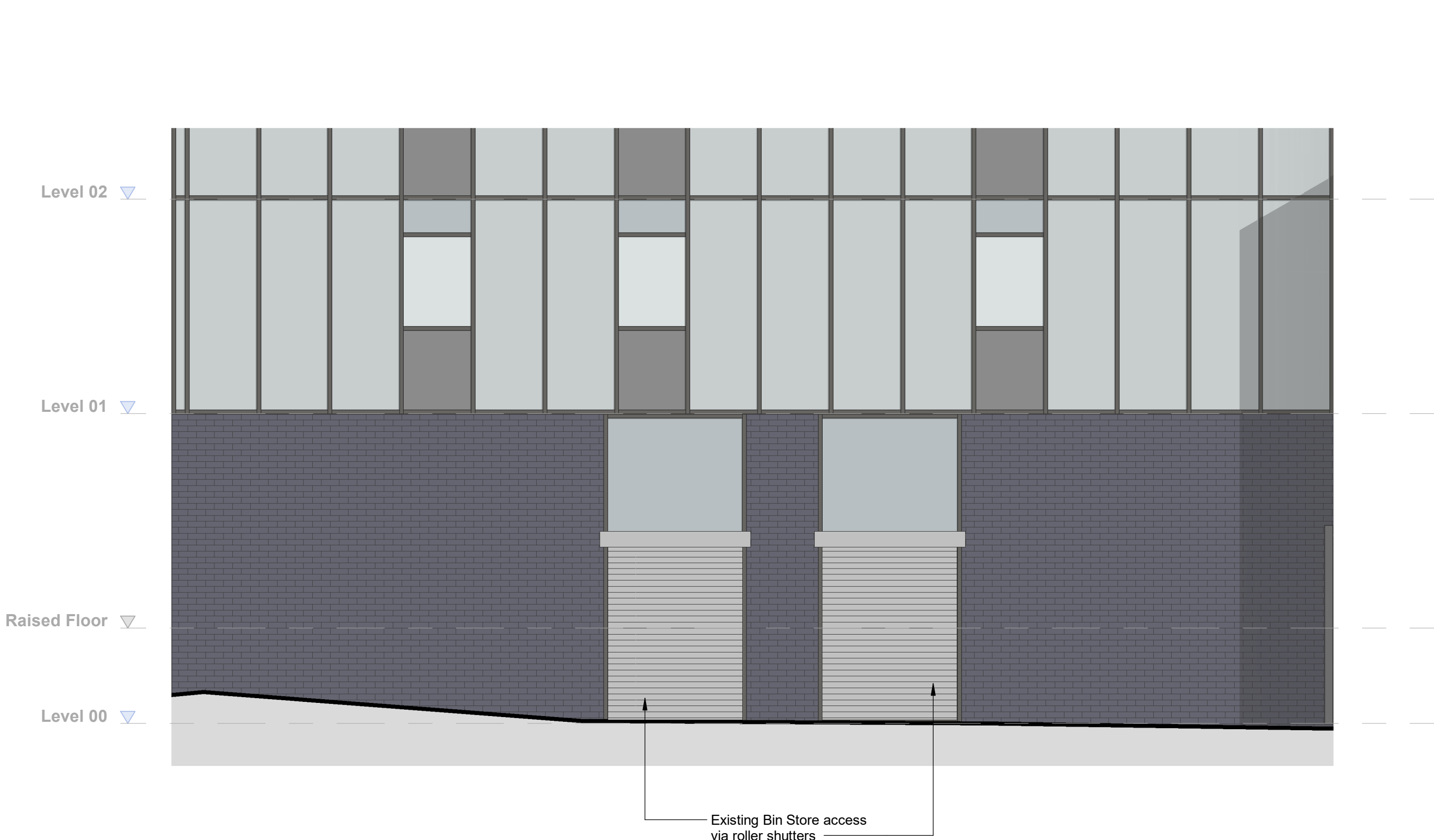
A Block 2 Existing Bin Store East Elevation 1 : 50
