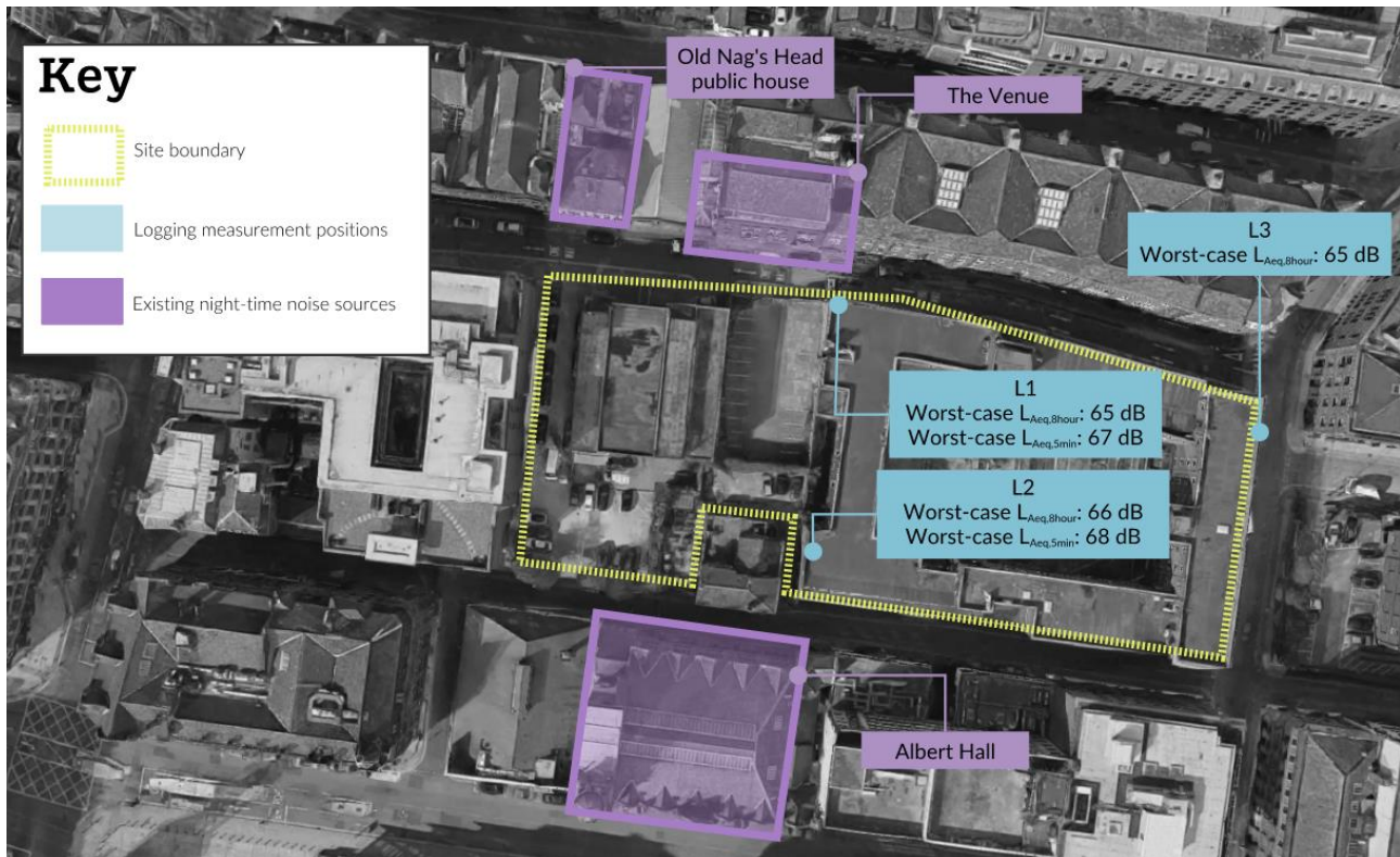
Figure A2 Annotated aerial image summarising measured noise levels captured during the night and key noise sources
