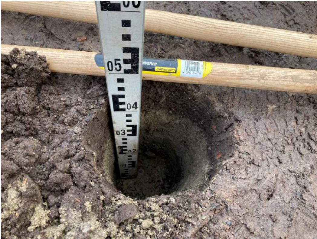
Photograph 7 VP04 showing 150mm of topsoil 400mm of subsoil.
