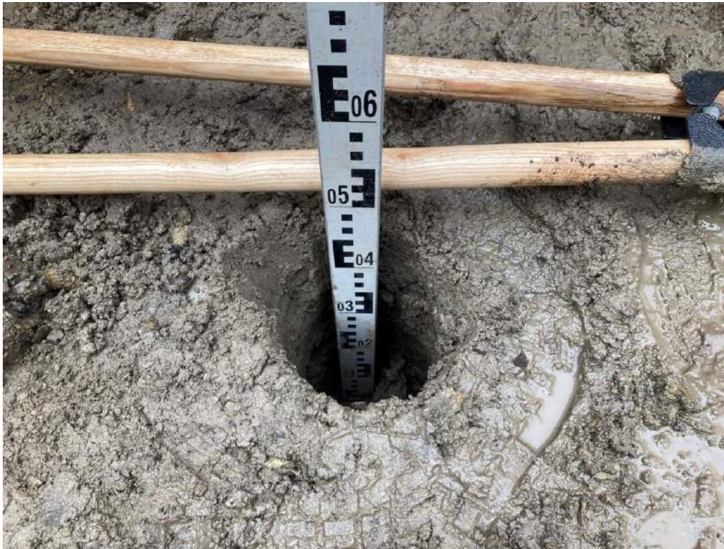
Photograph 3 VP02 showing 500mm of subsoil.
