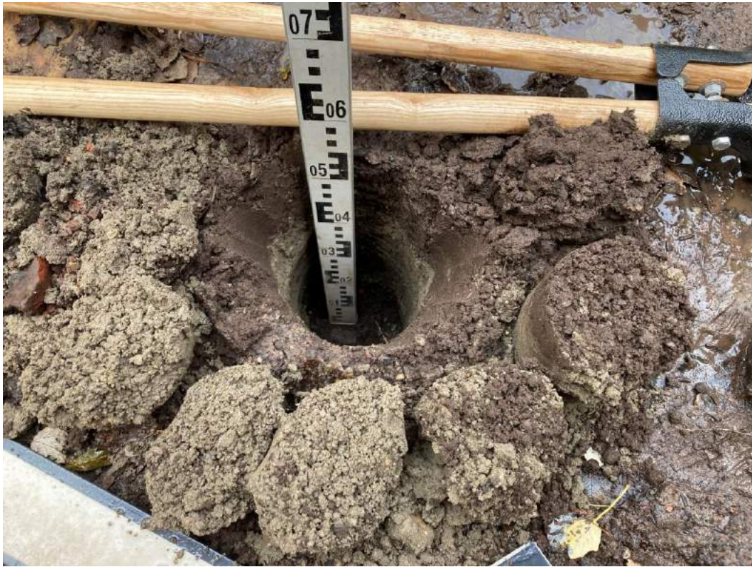
Photograph 1 VP01 showing 150mm of topsoil and 450mm of subsoil.
