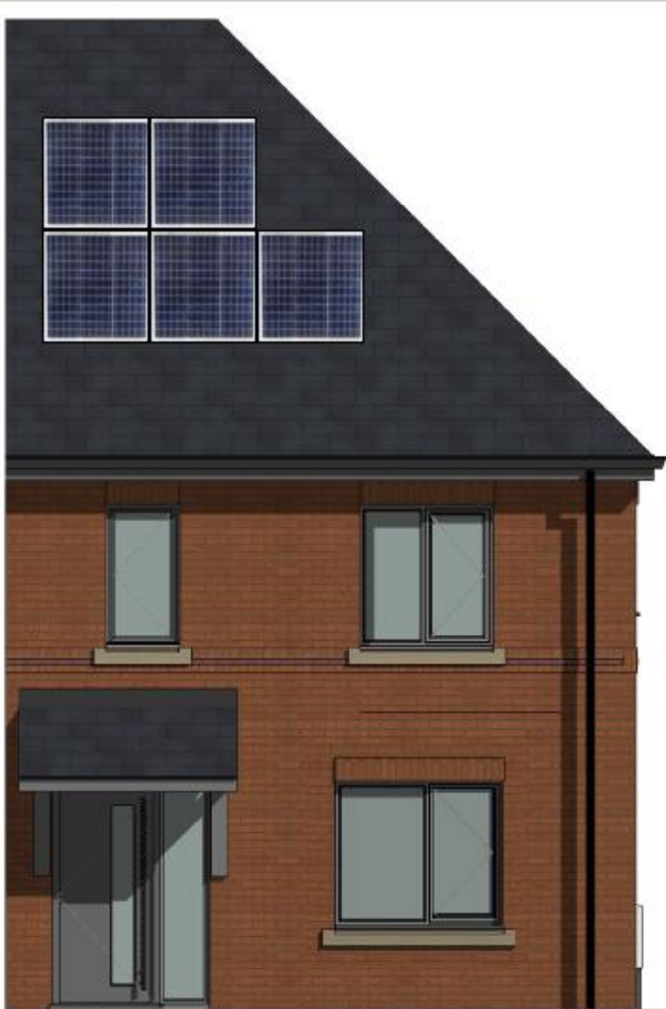
10 Front Elevation Brick Type A Hipped Roof 1 : 50
