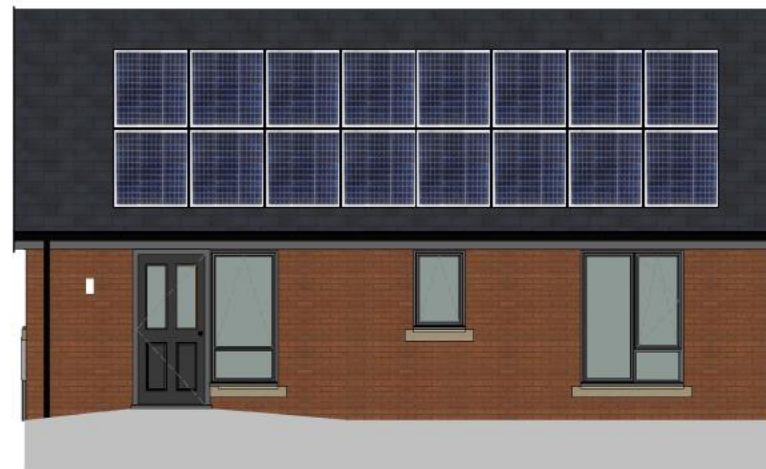
02 Rear Elevation Brick Type A Pitched Roof 1 : 50
