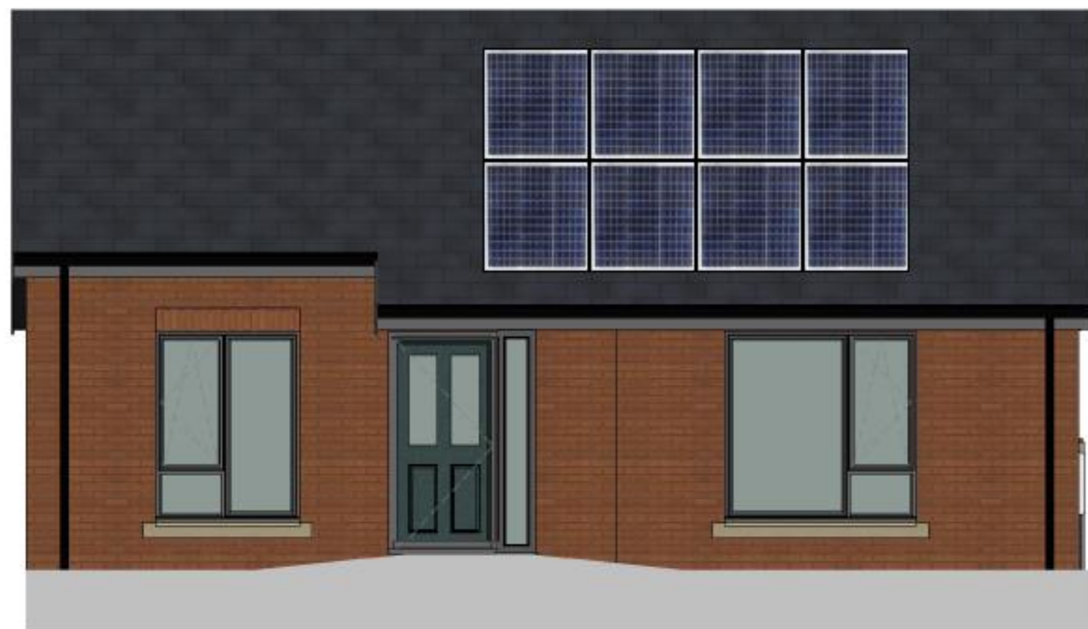
01 Front Elevation Brick Type A Pitched Roof 1 : 50
