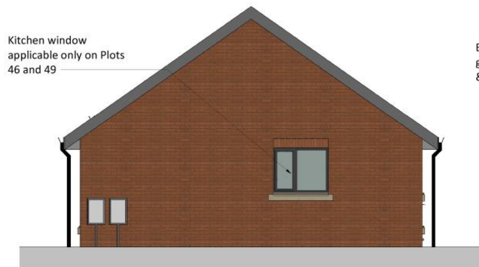
03 Gable Elevation Brick Type A Pitched Roof 1 : 50
