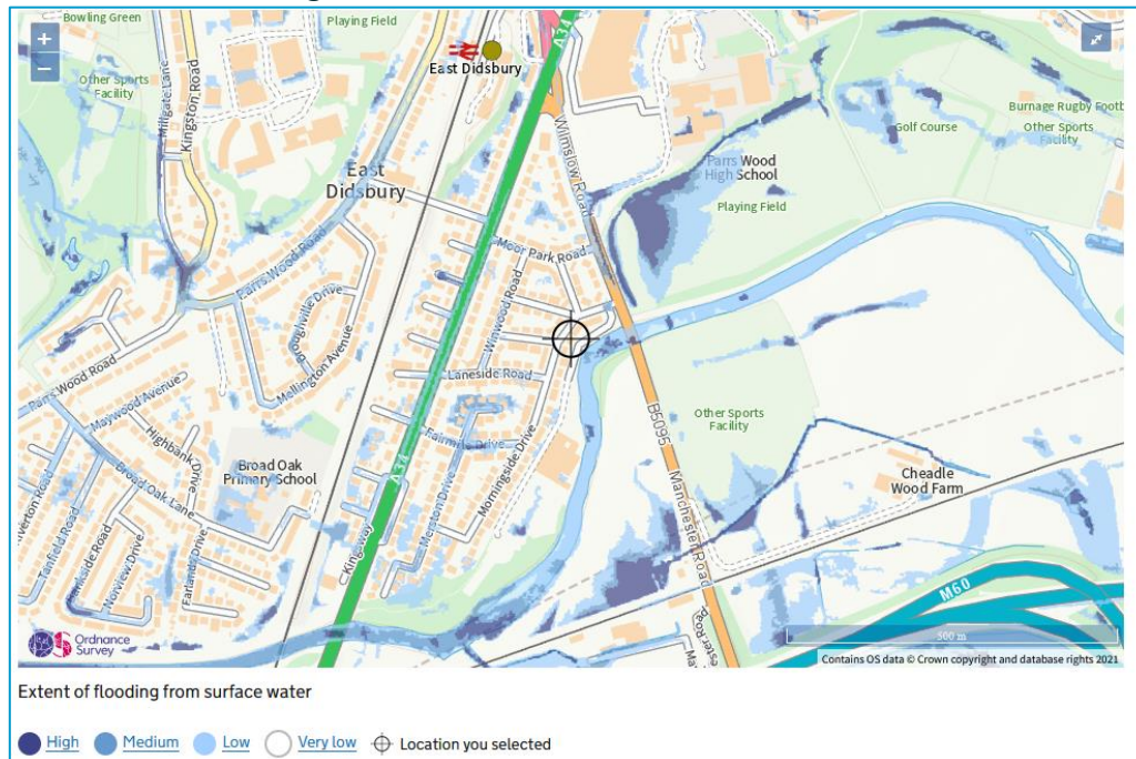
Figure 4.3: Flood Risk from Surface Water
