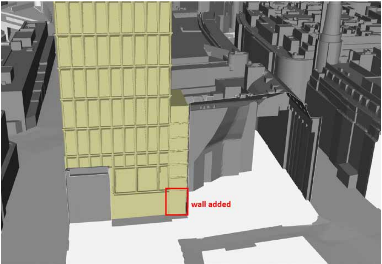
Fig. 09: Wall Added as Wind Mitigation
